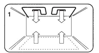
1. **Conventional Heating (Top Oven)** - with upper and lower heat. This system is particularly suitable for roasting and baking on one shelf only.
